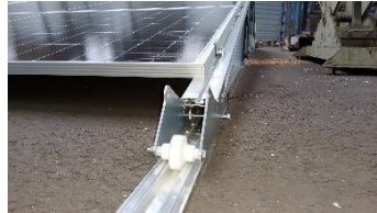
. 4 arrangement roller guides Fig
