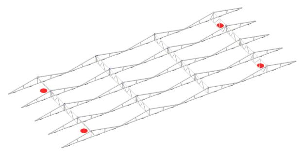
To easily install the roof anchors, it is possible to tilt the center in such a manner it doesn't obstruct the installation of the roof anchors. Tilt the centers at the locations of the anchors and mount the anchors.
