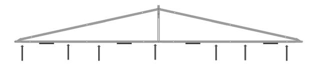
Additional feet can be placed on the positions of arrows.
