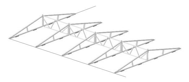
To extend the field in the column (X) direction, unfold the side and connect using the premounted connecting pin. Unfold the retaining clip and remove the connecting pin, slide the side connection plates to the previously installed sides. Slightly fold the connecting plates of the new side inwards and reconnect the connecting pin.
