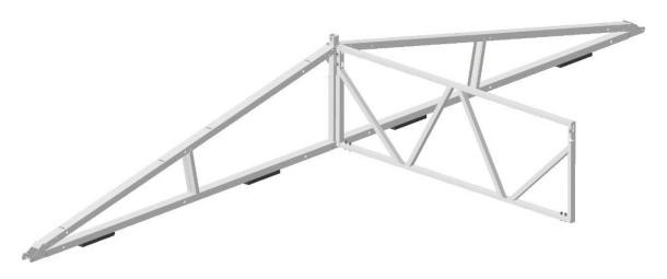
Repeat the unfolding procedure of the side as described before and attach the second side to the center as shown in the previous step.
