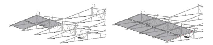
Follow the placement sequence of the panels as depicted below. The next step is the tensioning of the steel cable between the sides. Tighten the steel cable using the extended 13 mm socket (Article number 20-060-0033) with a torque of 20-25 N\*m. To prevent the steel cable from spinning while tightening, use the provided wrench (Article Number 20-060-0034) or a plier. To prevent friction welding of the stainless-steel nut and threaded end, lubricate the connection and tighten gently.
